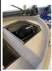
A lot of the time the petrol tank and filter connections are also placed in this same engine closed well, the closed well will thus house the petrol tank, outboard engine and all relevant assembly fittings including filters and hoses. Such an installation thus has all the characteristics of a petrol inboard engine as the compartment is closed during sailing.
